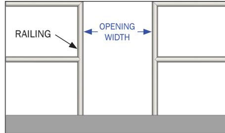
\*If bolting to angle iron, flat bar or wall surface, Adjustable Safety Gate opening width changes to 20 1/2" to 38 1/2".
